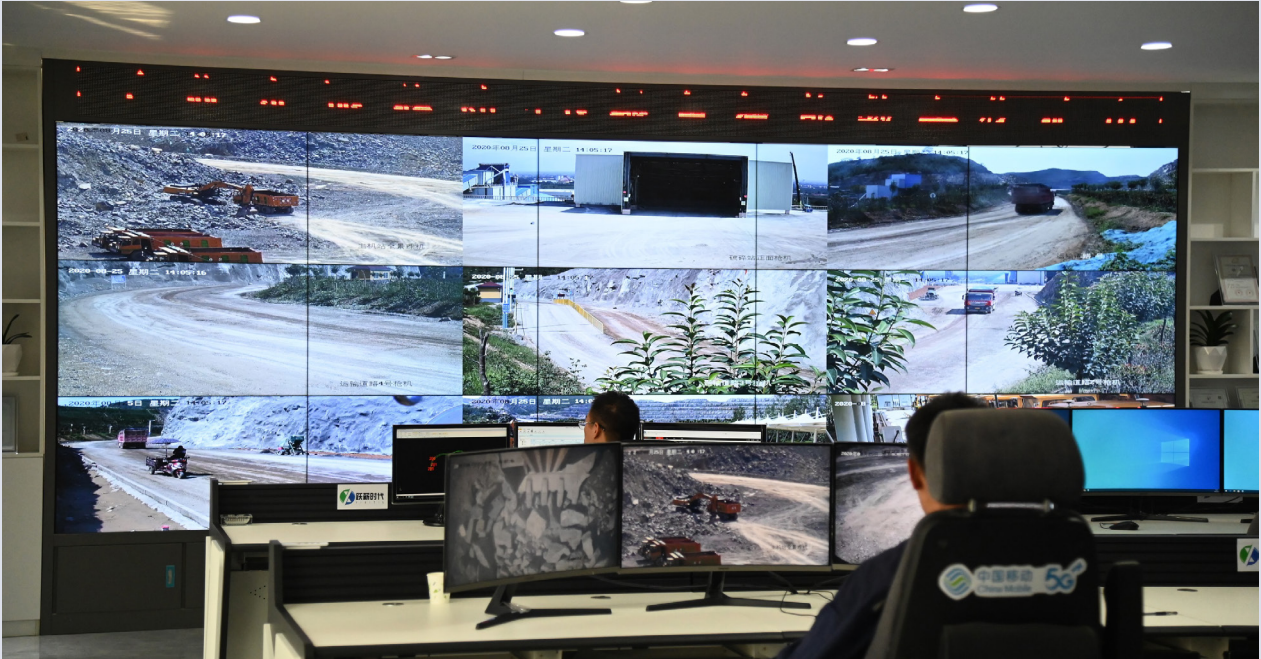
This is the intelligent dispatch center of Qianye Cement Company of Jiaozuo Coal Group, photo taken on August 25, 2020. Qianye Cement Co., Ltd. located in Jiaozuo, Henan Province, has used 5G network, Internet of Things, artificial intelligence cloud computing and other technologies to build a "5G+ unmanned mine" project to achieve unmanned remote control of mine crushing, excavation, transportation, monitoring and other aspects. (XINHUA)
